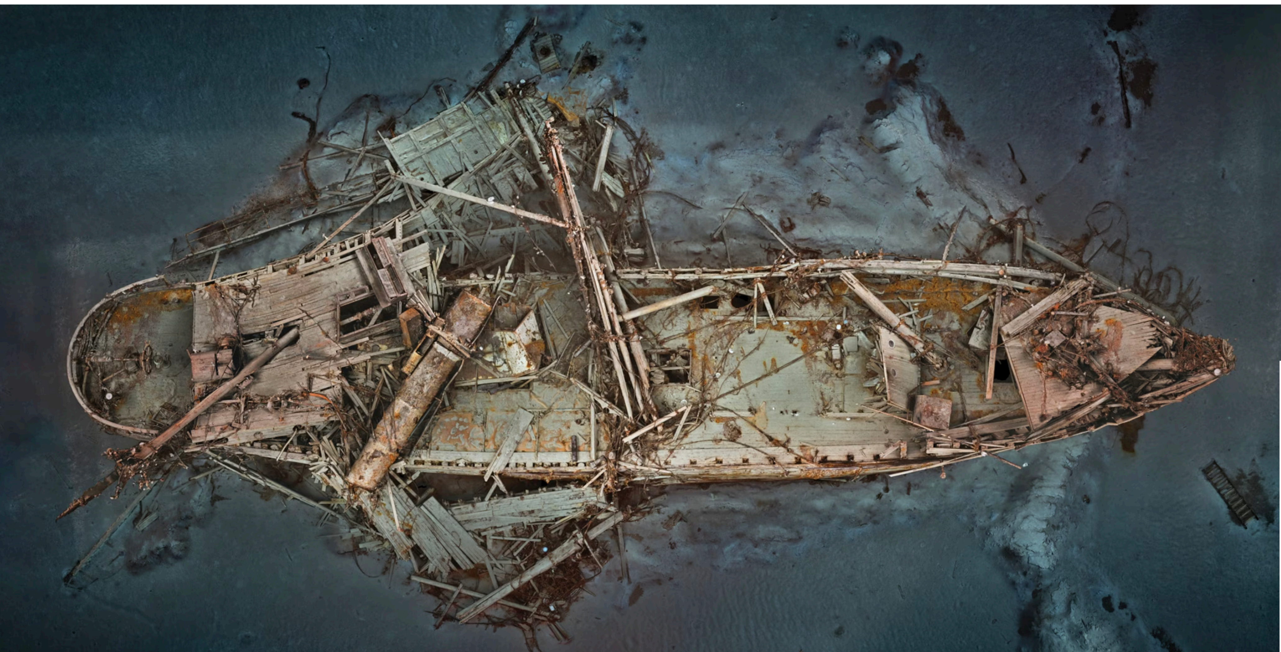
Twenty-five thousand photos in 4K resolution were used to create digital 3D photomosaics of the Endurance . Frigid, low-oxygen water helped preserve the wreck in pristine condition. COMPOSITE IMAGE BY THE FALKLANDS MARITIME HERITAGE TRUST
